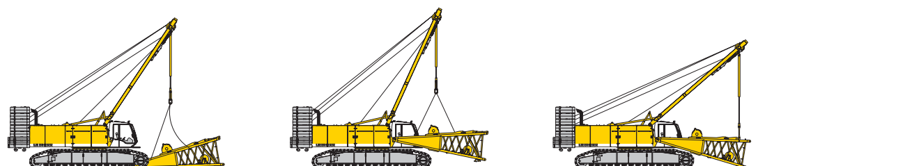
Unloading and assembly of boom foot
